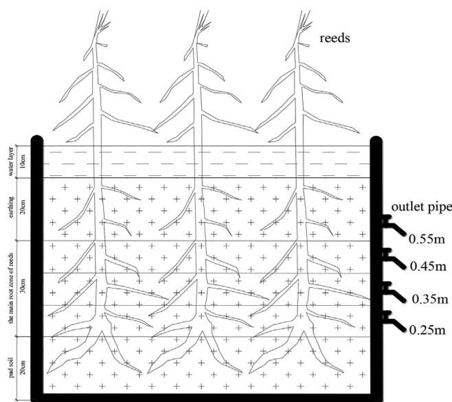
Fig. 1. The simulation device of reed wetland.
